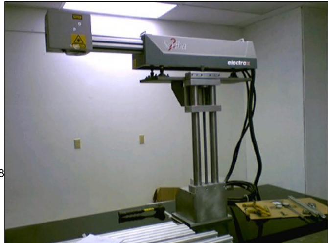
MS850Z series Z-Axis slide depicted with NEW Mounted Laser Application.
